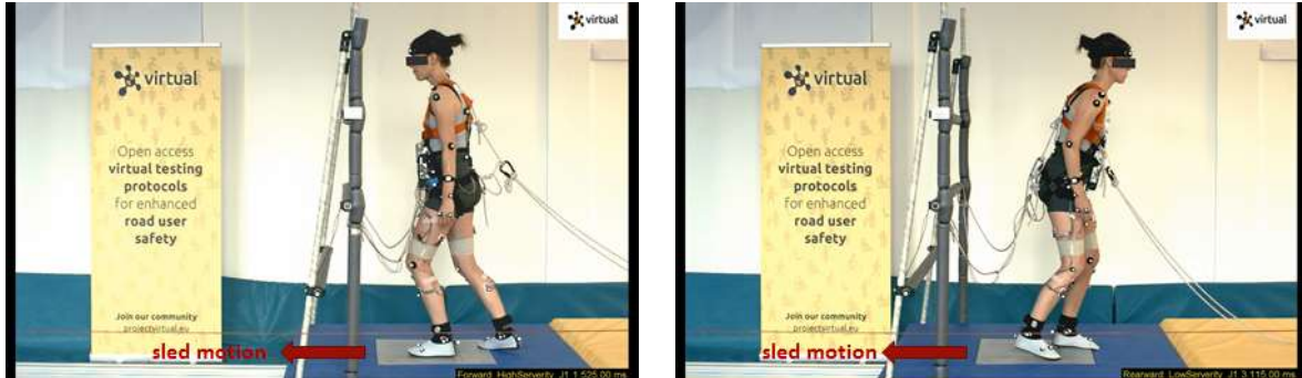
Figure 2-1: Forward and rearward orientation of the volunteers on the sled with the safety harness attached.
