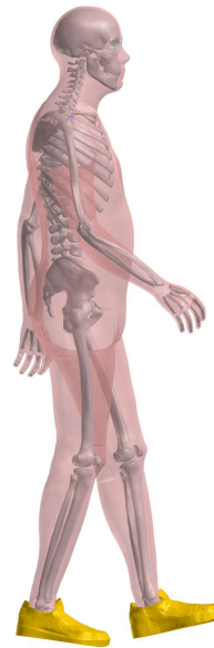
Figure 3-3: Positioned VIVA+ 50M model in accordance with the Euro NCAP Technical Bulletin TB024 (Euro NCAP, 2019).
