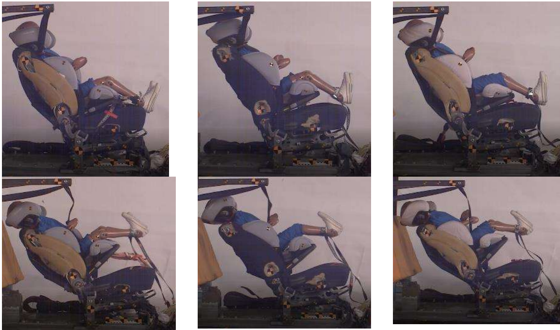
Figure J3. Snapshots of maximum vehicle seatback deformation for the booster seat in the headrest mid-position. Left to right. Top row, left to right: crash pulse 30km/h, T01 and T03 (booster seat version1), and T09 (booster seat version2). Bottom row, left to right: 50km/h, T02 and T04 (booster seat version1), and T10 (booster seat version2).
