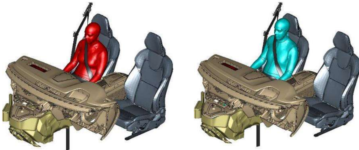
Figure 3-16 VIVA+ 50F (left) and 50M (right) seated in a front passenger seat in a vehicle interior model with nominal seat adjustment (25° seatback angle and 40% of the fore-aft travel).
