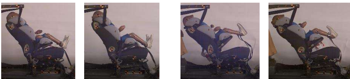
Figure J4. Snapshots of maximum vehicle seatback deformation for the booster seat in the headrest low-position . Left to right, crash pulse 30km/h (T05 and T07) and 50km/h (T06 and T08). An unintentional deformation of the rubber parts of the cap of the ATD's back head occurred, also resulting in a detachment in T06.
