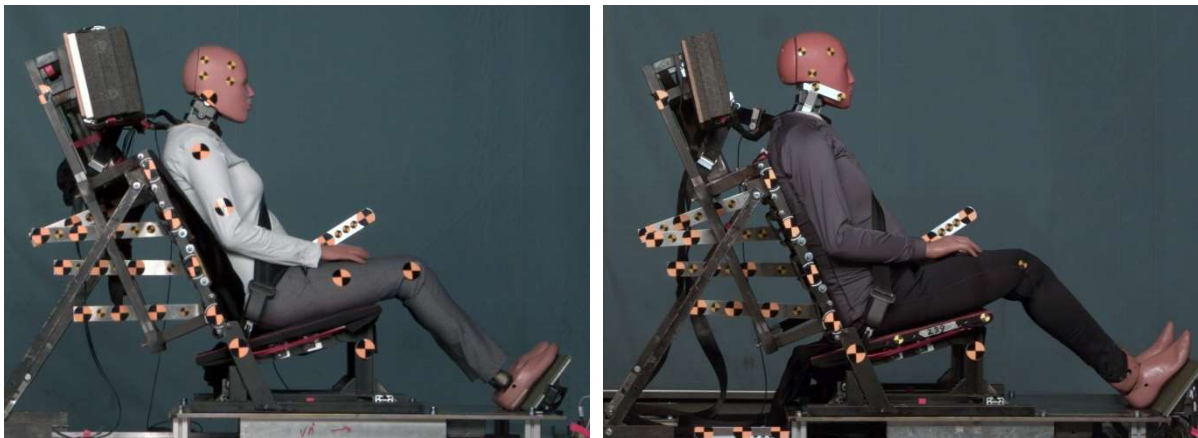
Figure 3-1 The SET 50F (left) and the SET 50M (right) seated in the Chalmers lab seat.
