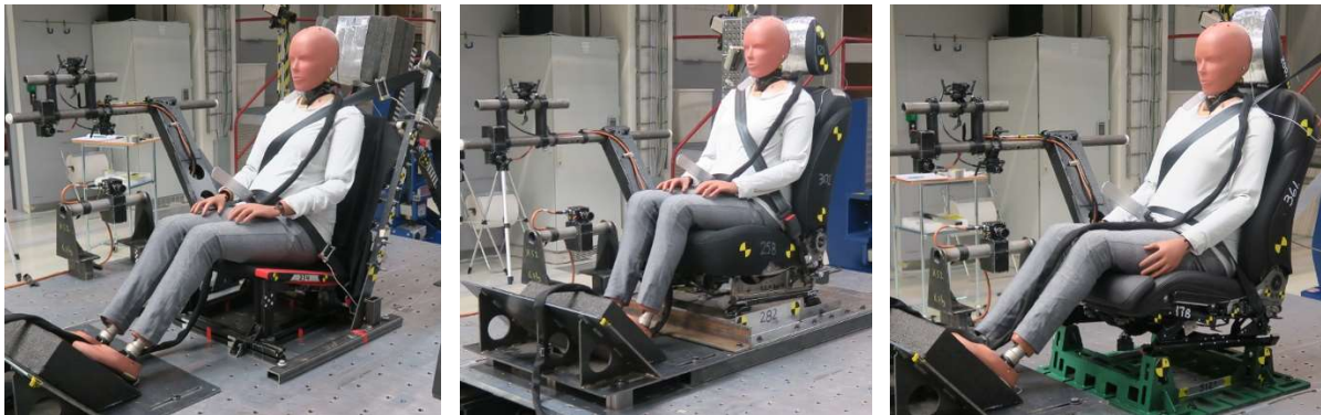
Figure 3-2 The three seats used in the study; Chalmers lab seat (left), Toyota seat (mid) and Volvo seat (right)
