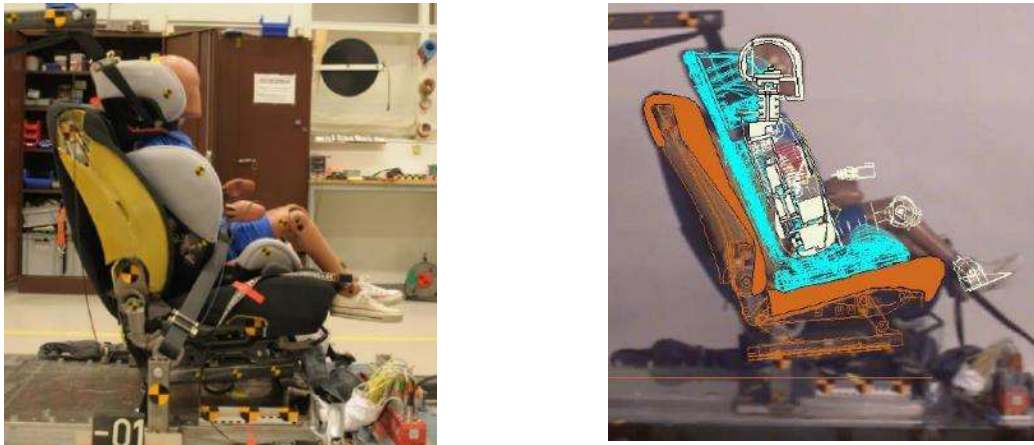
Figure 4-2 Sled test setup (left) and the corresponding numerical setup (right), booster seat headrest mid-position configuration and removed vehicle seat head-restraint. The vehicle seat is positioned rearward-facing in relation to direction of travel.
