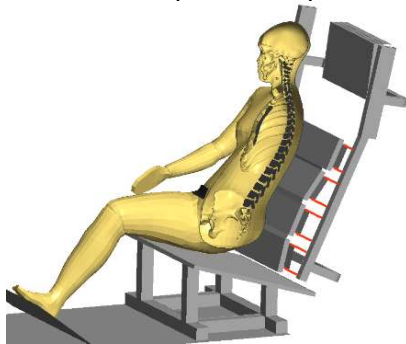
Figure E1. Oblique view of the simulation setup with the Chalmers lab seat used in this sub-study, and the VIVA+ 50F. Only the right half of the VIVA+ 50F is visible.
