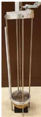
Figure A15. The impactors used in the physical tests. Impactor 1 was used in a drop test while Impactors 2, 3 and 5 were used in a pendulum setup.
