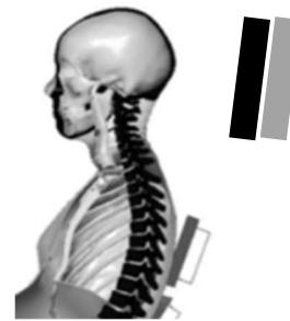
Figure E2. The two simulation setups, showing the two head to head-restraint distances of 100mm and 150mm.
