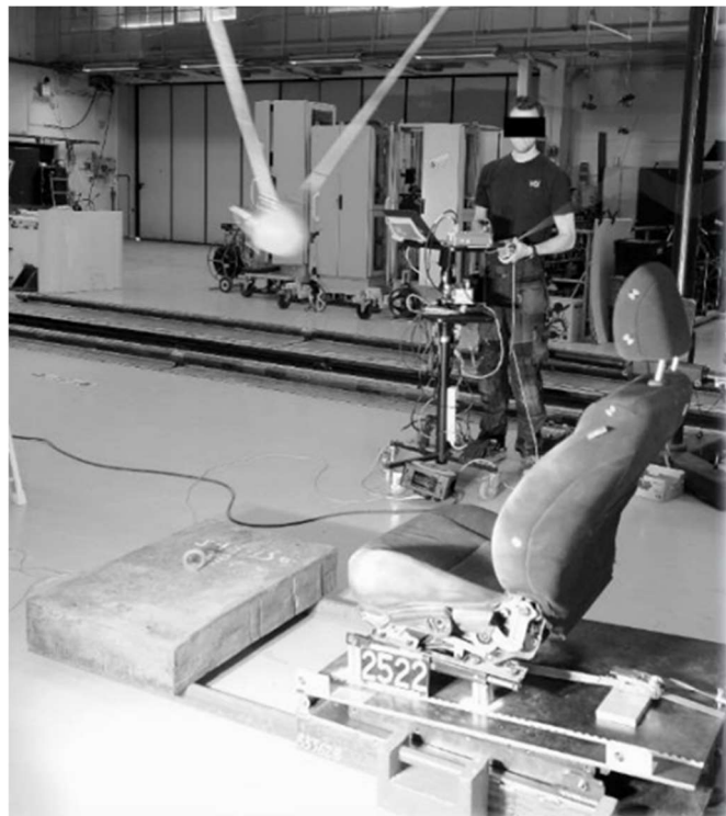
Figure 2-4 Pendulum test setup for test with Impactor 3. The seat is attached to the 'mousetrap'
