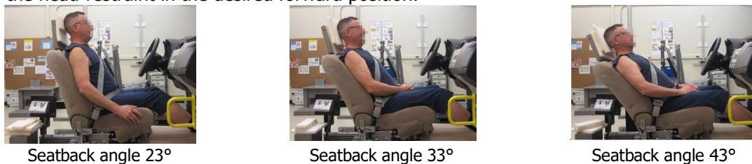
Figure 3-13 Posture study by UMTRI (Reed and Ebert, 2018), showing occupant's head position preferences when reclining the seatback.
