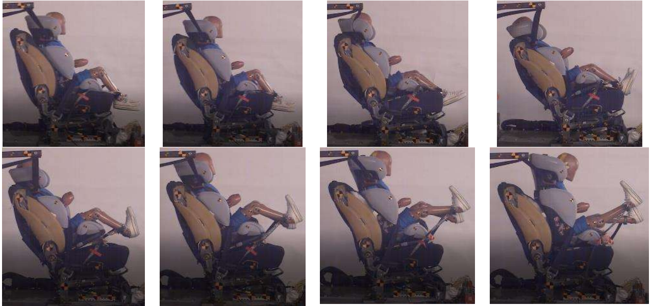
Figure 4-6 The sled test sequence from test T01; HIII6y with headrest in mid-position, exposed to a 30km/h frontal impact pulse (from left). Sequence starting top left (start of impact) to top right (maximum seatback deflection), followed by bottom left to bottom right (the rebound phase).
