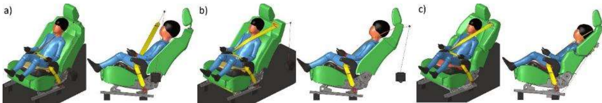
Figure 4-11 Seatbelt routing in the reclined position for a) V1 seat, b) V2 seat, c) V3 seat.
