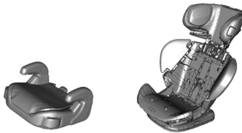
Figure 4-1 The two booster models used; booster cushion model (left) and OS booster seat model (right).
