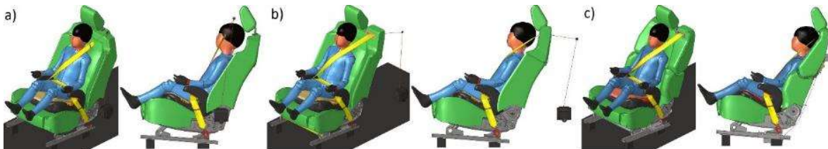
Figure 4-10 Seatbelt routing in the upright position for a) V1 seat, b) V2 seat, c) V3 seat.
