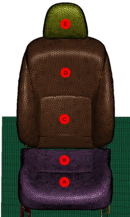
Figure 2-3 The VIRTUAL OS Vehicle seat model, including impact locations (a-e) in the validation study
