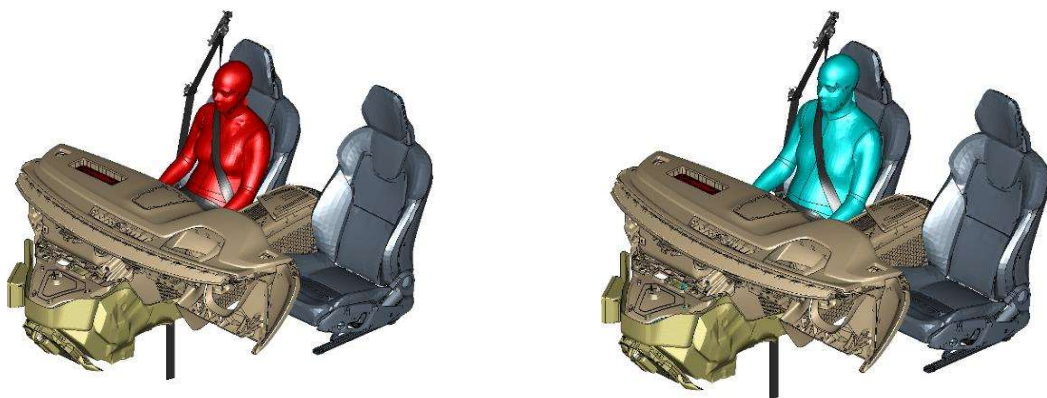
Figure I1. VIVA+ 50F (left) and 50M (right) HBM seated in a front passenger seat in a vehicle interior model in the nominal seat adjustment (25° seatback angle and 40% of the fore-aft travel).
