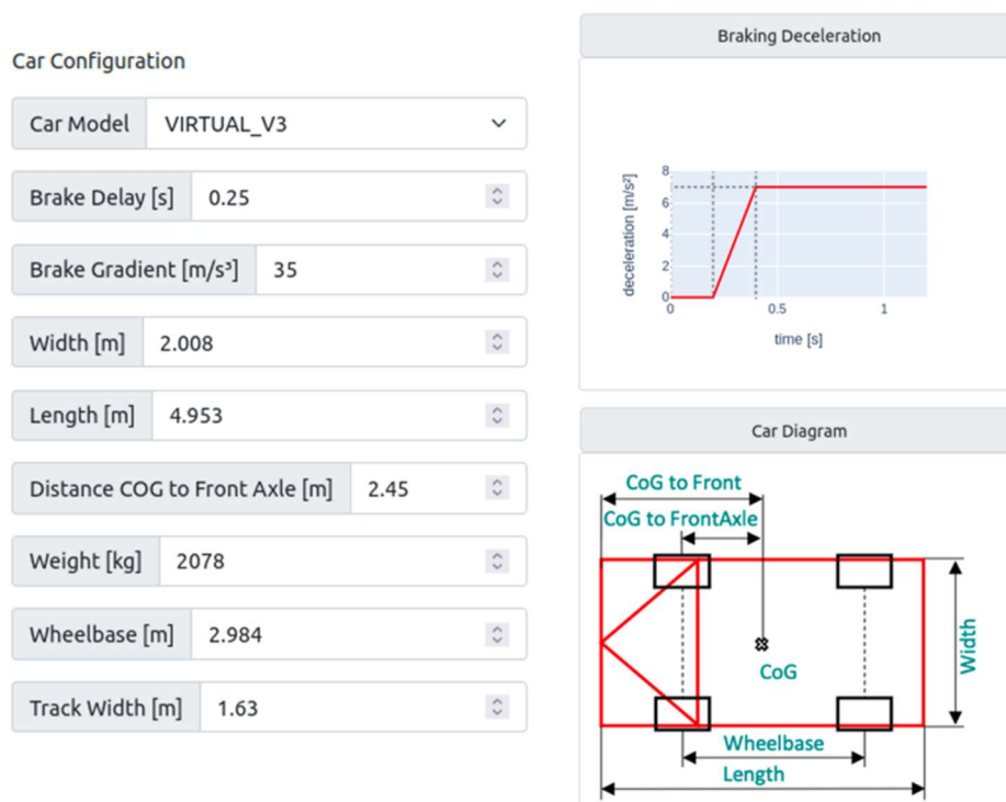
Figure 9-9: GUI for the car configuration with visualisation of configurable parameters (right) and interactive fields in which these parameters can be altered (left)
