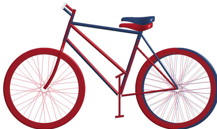
Figure 9-14 Overlay of bicycle for VIVA+ 50F (trapeze frame; red) and VIVA+ 50M (diamond frame; blue)
